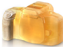
Fig. 1.2. Stereolithography mock-up of a camera with Balsa wood grip.
