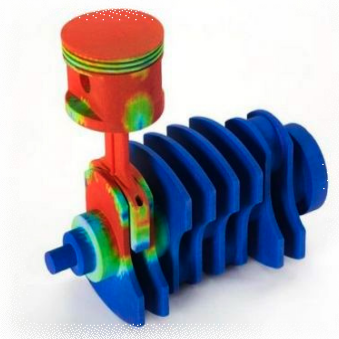
Fig. 1.1 Thermal model of a piston and crank shaft assembly.
